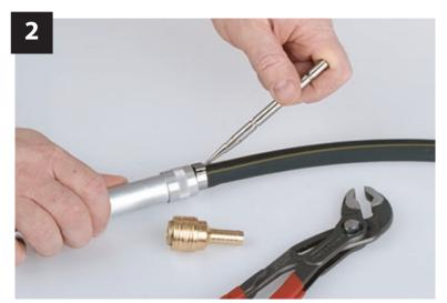
Use a screwdriver or a sharp tip to loosen the hose clip and pull out the hose.
