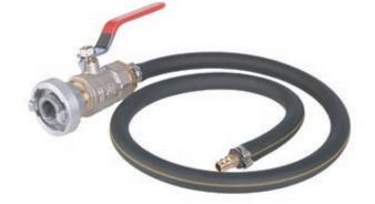
The filling system is connected to the water source via a D coupling. The filling hose is terminated with a quick-connect coupling's plug, just like the end of the handheld pump of the firefighting backpack. The firefighting backpack is equipped with a quick-connect coupling at the end of its hose for quick switching between filling and handheld pump. Therefore, no assist is required for filling. The quick-connect coupling is one-way - no water will leak out of the backpack when unfastened.
